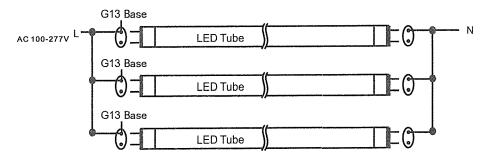
Fourth Step: Affix the field applied label to the light fixture. Then install the tube. The tube is double port wiring connection
