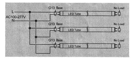
Fourth Step: Affix the field applied label to the light fixture. Then install the tube. The tube is single port wiring connection
